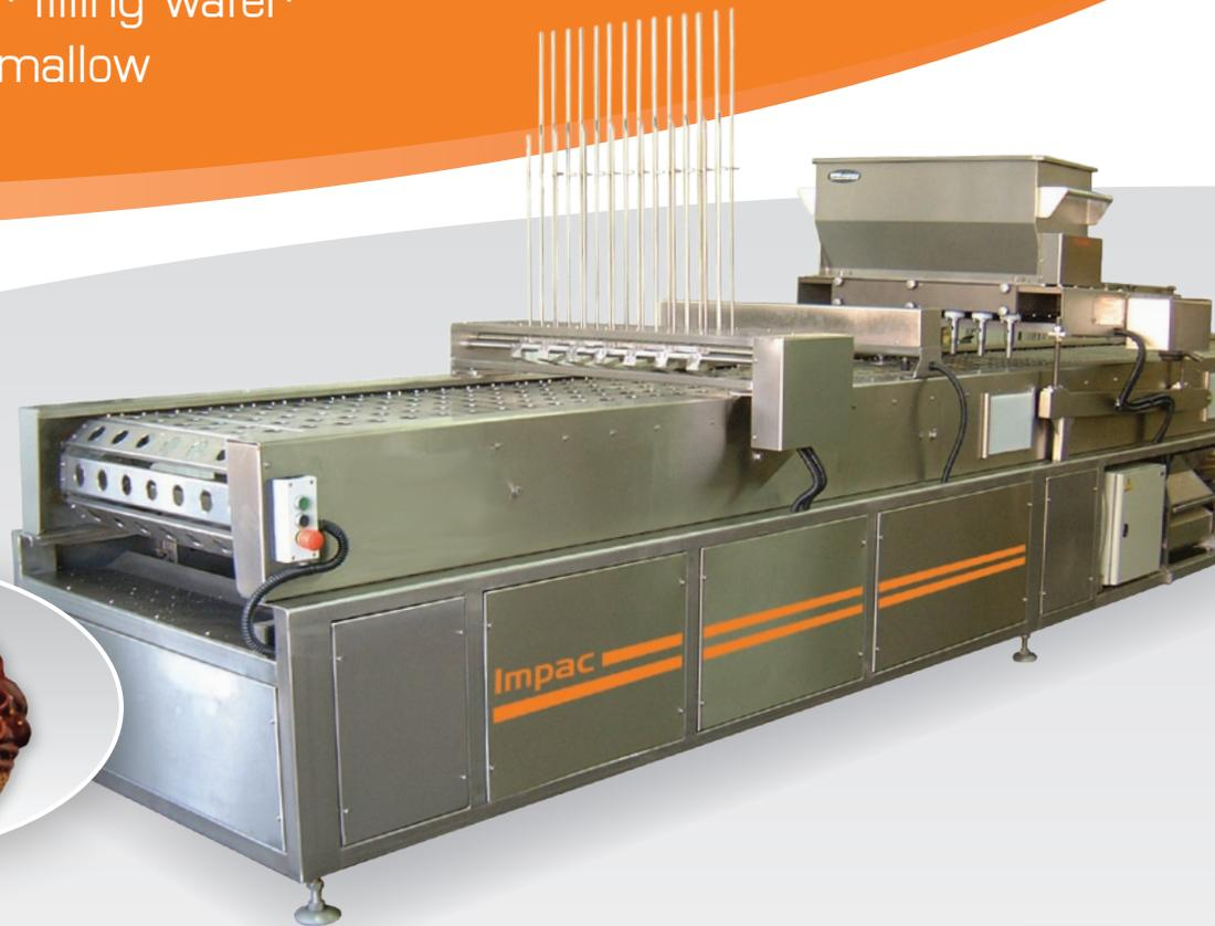
The machine is suitable for filling homogeneous Albumin foam (marshmallow) into wafer cones and coating them with chocolate. The machine includes the following systems:
